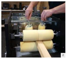
Adjust the sponges to the dimensions of the element and fix them by tightening screws.
