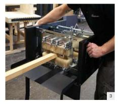
Adjust the brushes to the dimensions of the element and fix them by tightening screws.
