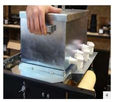
Position the colour tank and make sure that nozzles are closed. Hook the collection bucket under the tank.
