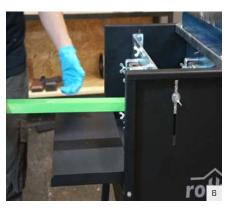
Start the process: open the nozzles and wait for the rolls to absorb the colour. Finally, push the elements through the sponges.
