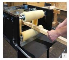
Insert the element between the two automatic coating machines
