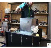
Enter paint or impregnating primer. If necessary, mix it until a homogeneous consistency is obtained.
